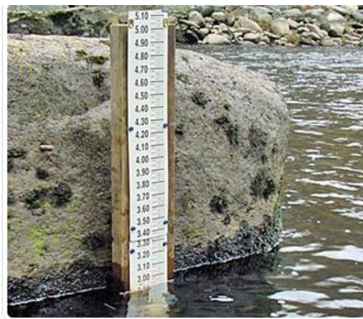
A Typical Arrangement Used to Measure Water Level. The water level records are used to obtain the stream flow values.
